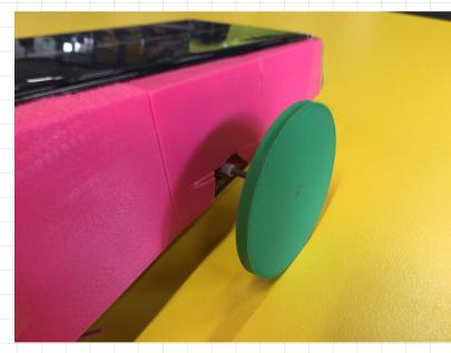
Another issue that was discovered with these plans was that I had not left a hole For the axke. The body was cut using side cutters and sealed using a soldering inon.
