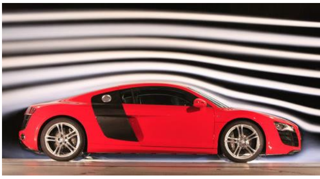
Figure 4 shows an Audi R8 in a wind tunnel showing how traces of wind move around the vehicle.
