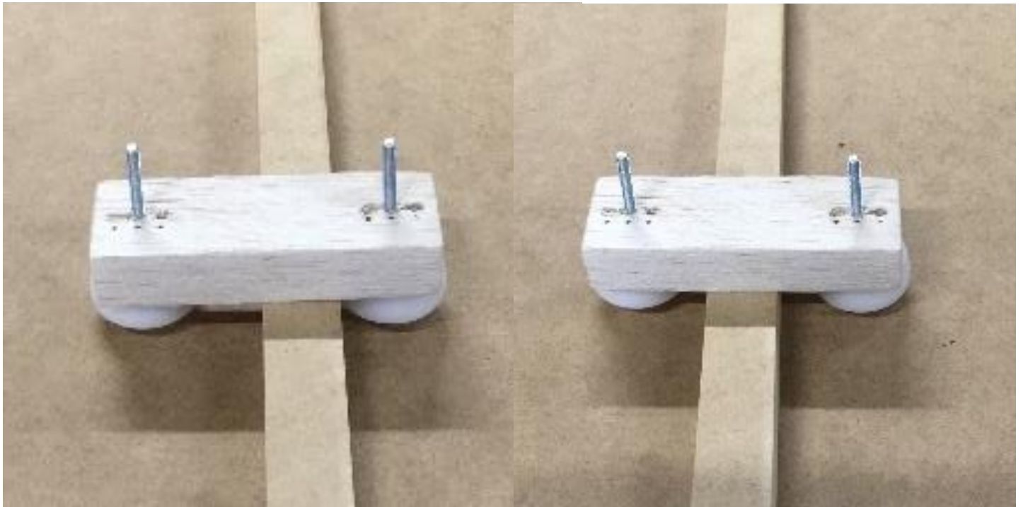
Figure 21: The Balsa guide wheels. Image on the left shows the guide wheels veering to the left with the right wheel in contact with the rail. The image on the right shows the guide wheels when perfectly straight.
