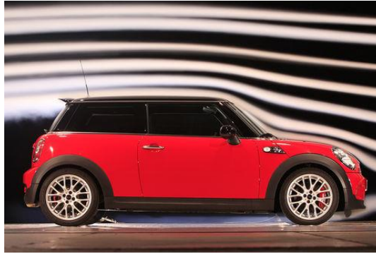
Figure 5 shows a Mini Cooper S in a wind tunnel showing how air moves around a more box like car compared to the Audi. It also shows a greater low-pressure area at the back of the car (The dark area where there's no air strands).
